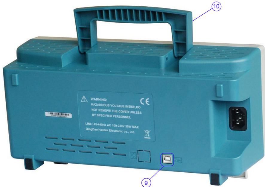
**9 USB Device Port Combined with PC** -- Easily communicate with other instruments, peripherals or system via usb. The USB port allows you full programmable controls for automated measurements and remote display and archiving.
